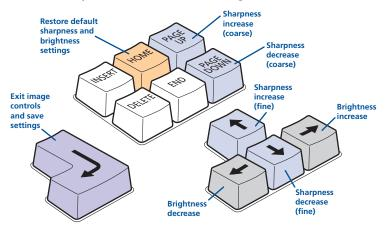
4 When no shadows are visible and the displayed images have crisp edges, press to exit configuration mode and permanently save all settings.
