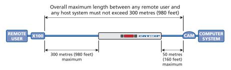
In situations where any computer system will be placed a significant distance from the AdderView CATx unit, ensure that the distance to any remote user is similary less than 300 metres (980 feet).
