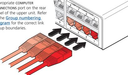
3 Connect the other end of the cascade link cable to one of the CATX USER PORTS sockets on the rear panel of the lower unit. Due to the way in which ports within a link group are dynamically allocated, it is not usually important exactly which user port is connected to each computer port of the upper unit.
