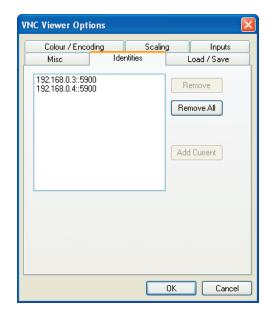
If an existing AdderView CATx IP is fully reconfigured then it will need to issued with a new identity. In this case the previous identity, listed in this tab, should be removed so that a new identity can be created on the next connection.
