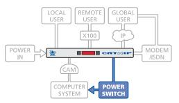
The control connector of the first power switch is attached, via serial cable, to the rear panel of the AdderView CATx IP. Any additional power switches are then attached via a 'daisy-chain' arrangement to the first power switch. Each power switch box is then given a unique address and access to each power port (8 ports on each power switch box) is gained using a combination of the switch box address and the port number.
