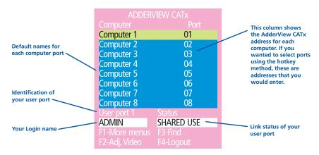
To view this menu at any time: Press and hold the hotkeys (usually  $\Box$ th), then press  $\underline{M}$  and finally release all three keys.
