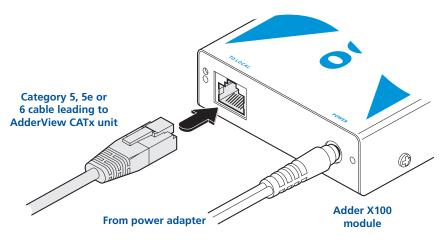
5 At the other end of the cable run, attach the cable connector to one of the sockets labelled CATX USER PORTS on the rear panel of the AdderView CATX unit.
