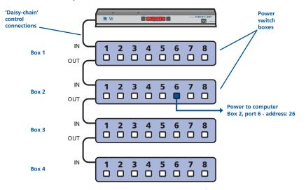
The power ports are connected to the power inputs of each computer system and the power switch box(es) are then connected to a mains power supply.
