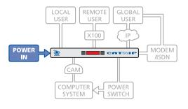
Note: AdderView CATx units require a heavy duty power adapter at either or both power input connectors. Use only the adapter supplied with the unit or available under Adder part numbers: PSU-IEC-5V4A (for AdderView CATx) or PSU-IEC-5V6A (for AdderView CATx IP). Do not use the standard 10W adapters that are supplied with other Adder products, such as the X100.
