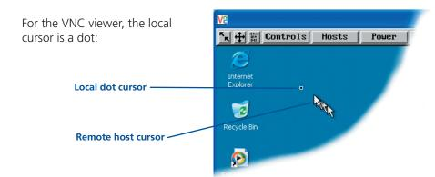
Additionally, for fast network connections, the VNC viewer also provides a single mouse mode. See <u>Controls - Single Mouse</u> for details.
