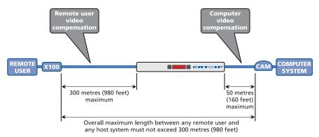
Note: For installations where both computers and remote users require video compensation, always ensure that the computers are compensated first.
