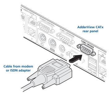
Note: The default serial port speed is 115200 and a standard Hayes-compatible auto-answer string is sent during startup. The default startup string is 'ATZHS0=1'. Both the serial port speed and startup string settings can easily be altered during configuration - see <u>Initial IP configuration</u> for more details. The other serial settings are fixed at: No parity, 8 bit word and 1 stop bit.
